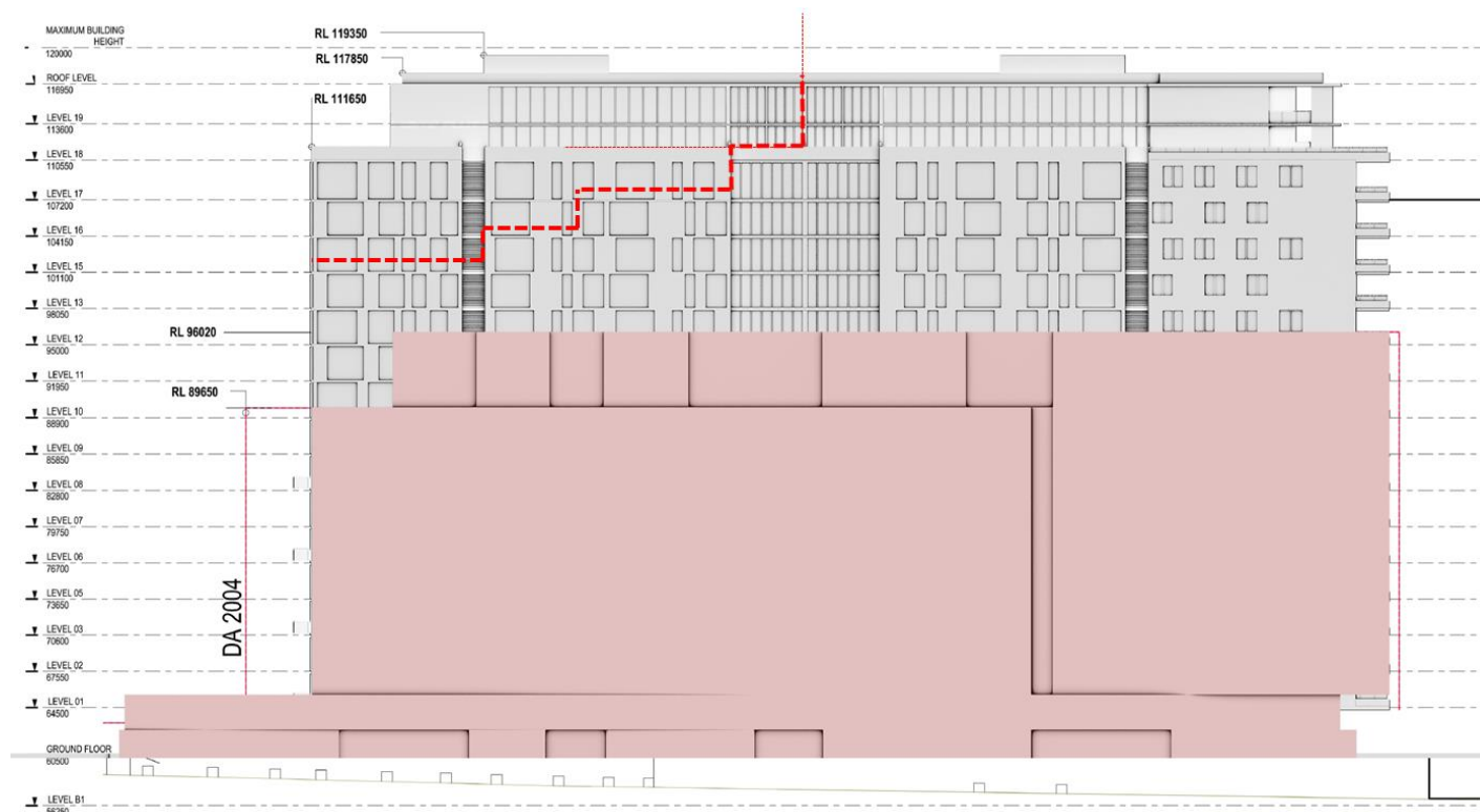
Figure 3: Diagram illustrating reductions necessary to achieve target 3 hour compliance for 504 Railway Pde on June 21 and 3-hour compliance for 1-3 Noble St on no less than 300 days
